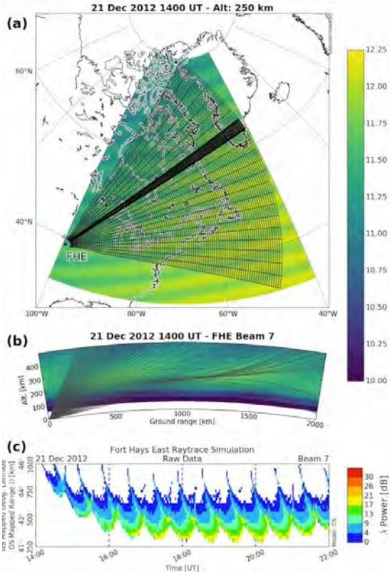
Ray trace simulation illustrating how SuperDARN HF radars observe MSTIDs.
