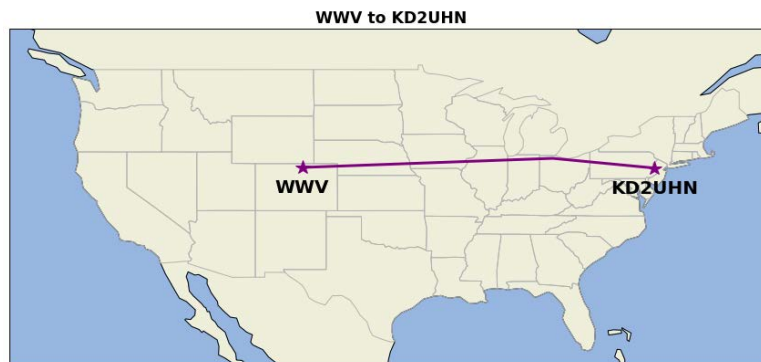
(FIGURE 2) The map shown above depicts the path traveled by radio waves transmitted by WWV (left) and received by KD2UHN (right). Notice, due to the distortions of a 2-Dimensional map, the radio wave does not propagate in a straight line on the map, so the Great Circle Path appears curved. This map was generated using cartopy in the Python language.
