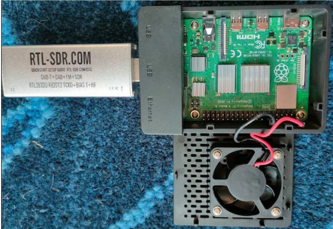
Pictured above: Our RTL-SDR connected to our Raspberry Pi with heatsink.
