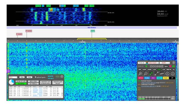
Fig. 8: WSPR signal left of ZSRF is a non-decode at SNR -27 dB at KiwiSDR in Philippines and will not be stored in WSPR database
