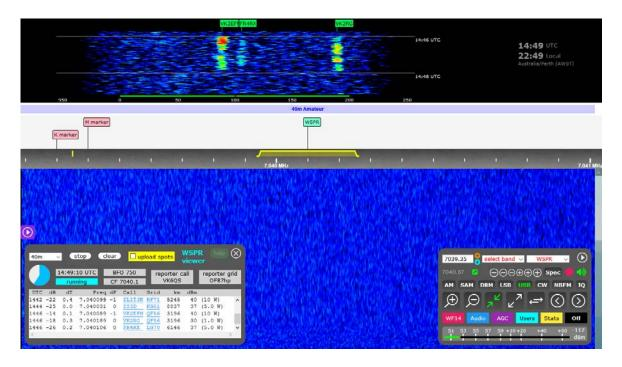
Fig. 2: Strong blip on shape of WSPR signal VK2EFM at screen of KiwiSDR at VK6QS in Perth, Western Australia
