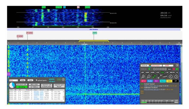
Fig. 6: Non-decode with SNR -27 dB at app. 150 Hz in WSPR band left of JA5NVN will not appear in WSPR database
