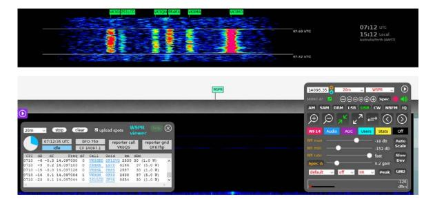
Fig 1. : WSPR waterfall from VK, FR, ZS signals on screen of KiwiSDR at VK6QS in Perth, Western Australia
