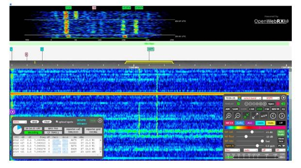
Fig. 7: Bi-/Multilateral reception of WSPR signals in Indonesia and Philippines enables identification of WSPR signal HS2JFW at SWLO133 close to Jakarta / Indonesia as well as close to Negros / Philippines. This information will be lost in WSPR database (www.wsprnet.org)
