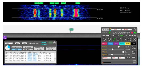
Fig. 3: Very strong WSPR signal of VK3MO due to aircraft scattering at RX VK6QS in Western Australia (Perth)
