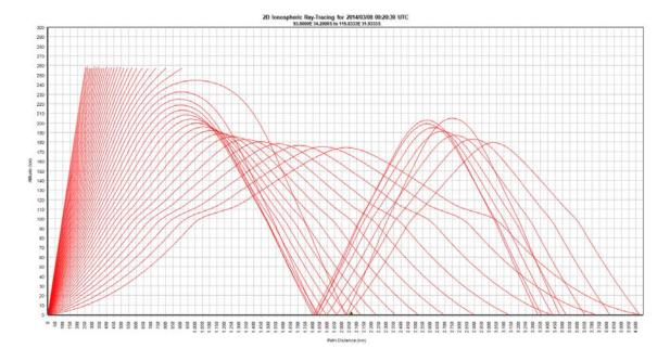
Fig. 33: Ray tracing between IG LEP and VK6ZRY in Perth (Proplab 3.1)
