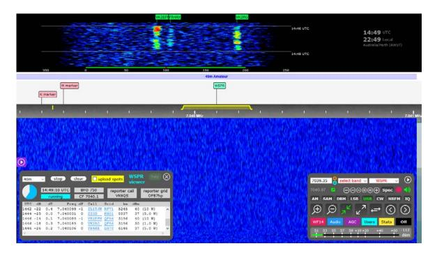
Fig 4.: VK2EFM WSPR signal shape deformation at drift -1 Hz/min due to scattering. FR4RX signal from Réunion as well as VK2RG not effected with drift 0 Hz/min.
