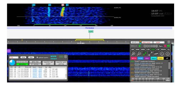
Fig. 10: Strong nondecode with "odd shape" of WSPR signal due to drift > -4 Hz/min
