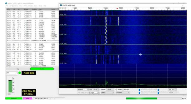
Fig. 15: WSPR signal of French WSPR station in Bretagne deformed to a "snake" in WSJT-X probably due to air scatter between two aircraft
