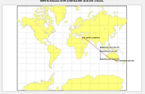
Fig. 31: Midcourse WSPR detection between RX 4X1RF and TX VK3DXE at 21:20 h UTC matched to Inmarsat data (Graphics courtesy of Richard Godfrey)
