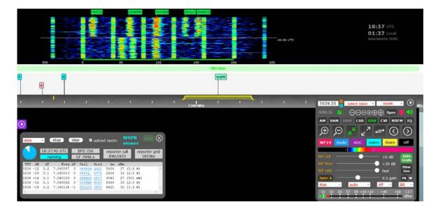
Fig. 16: Numerous WSPR signals received by SWLOI33 in Indonesia with interference by OTH Radar
