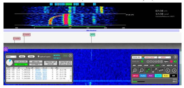
Fig. 11: WSPR Signal with very strong deformation due to air scatter (non decode) probably due to strong banking of aircraft after departure from MEL in Australia.
