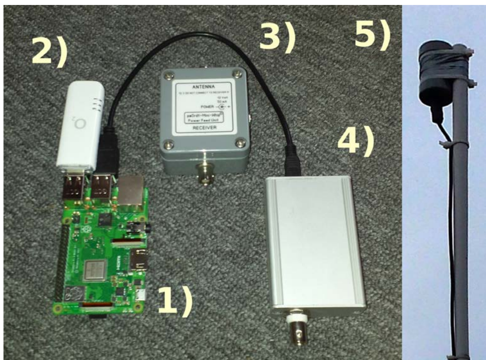
Figure 5: The PAORT Mini Whip active antenna is an electric field active antenna in a small package (Figure 5.5.) This antenna type has been selected as the 'perfect' fit for our broadband VLF SID monitor (private Communication with Mr. Roelof Bakker). It is connected with a "Power Bridge" (Figure 5.3) to the SDR.
