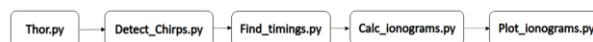
Figure 3. The steps involved in data collection and execution of the Chirpsounder2 software package.
