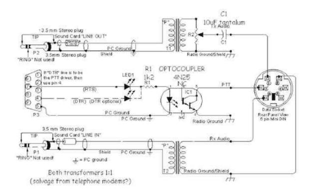
You may not need the PTT part of the circuit as most rigs support PTT by computer control through the USB or serial connection. The source of audio and PTT may cause some confusion: Some rigs, if keyed by PTT in the AUX or DATA connector take the audio input only from the AUX connector, and not from the mic connector.
