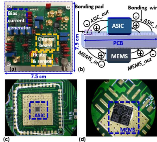
(a) Test PCB. (b) MEMS and chip integrated into the PCB. (c) Wire-bonded chip on the PCB. (d) Wire-bonded MEMS on the PCB.
