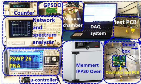
Experimental setup for testing the MEMS-based GPSDO.
