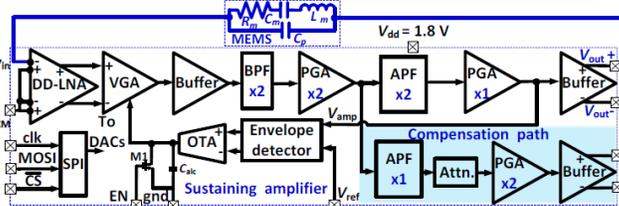
Block diagram of the MEMS resonator and chip.
