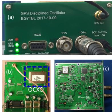
(a)-(c) Commercial GPSDO used for injection locking the MEMS-based oscillator: (a) front view, (b) top side of PCB, (c) bottom side of PCB.
