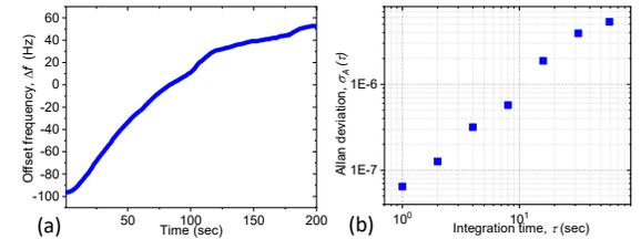
(a) Time-frequency data (b) Allan deviation of MEMS oscillator only.
