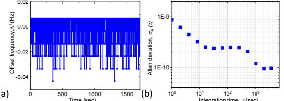
(a) Time-frequency data (b) Allan deviation of MEMS-based GPSDO.
