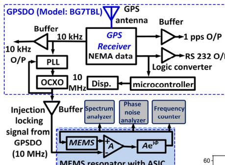
Overall architecture of the GPS-disciplined MEMS oscillator.
