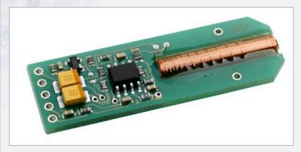
Complete miniature fluxgate magnetometer can be used in any application where the sensitivity of Hall- or MR-magnetometers is not sufficient, e. g. measurement of the earth's field, detection of AC field from power lines, vehicle detection, compass navigation, and many others. Due to its low price and low power consumption ideally suited for multi-sensor array systems.
