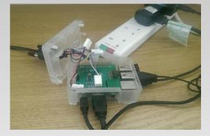
"Raspberry Pi Magnetometer" by British Geological Survey (BGS)
