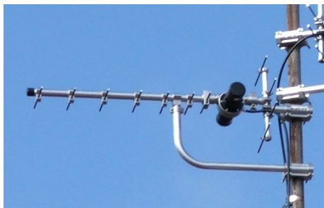
Fig. 1. The 12 elements UHF Yagi-Uda antenna.
