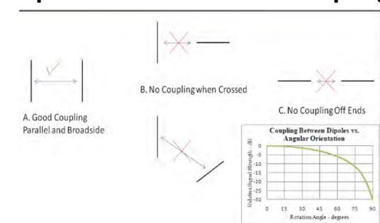
Fig. 4: Dipole Orientation and Coupling. Reprinted from Cerwin (2019).
