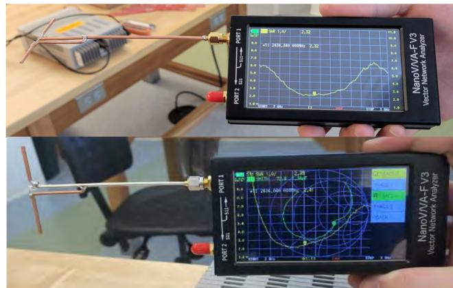
Fig. 2: Matthew Dittmar's dipole antenna being tested using a NanoVNA.
