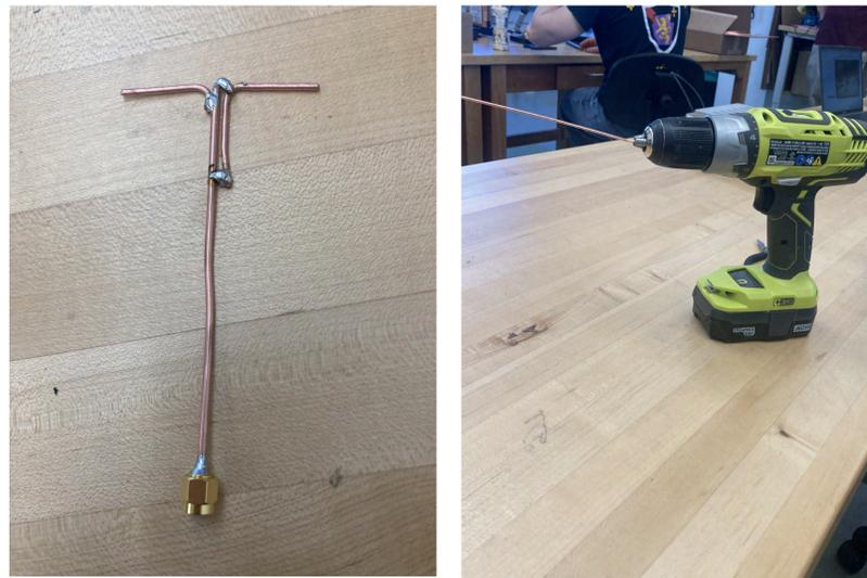
Fig. 1: A) Completed dipole antenna with superb soldering job. B) Steve Cerwin's pro-tip to straightening and strengthening copper.
