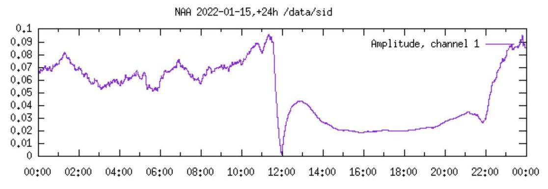
In this plot of NAA above captured at the Springbrook Township, PA, US, at 5:00 UT, a noticeable reduction in signal amplitude can be observed. This could be caused by either a Sudden Enhancement of Atmospherics or a perturbation of the ionosphere along the propagation path due to the eruption's pressure wave.
