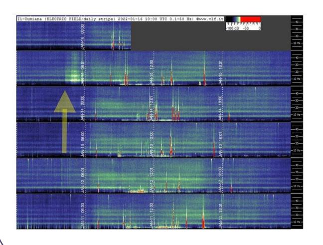
The image on the left (credit to Renato Romero IK1QFK) are stacked spectrogram plots of the Schumann resonances, or the resonant modes of the Earth-ionosphere waveguide. These resonant modes are in constant excitation due to worldwide sferics. At around 5:00 UT as shown by the arrow, an intensity in excitation can be observed due to the SEA created by lightning from the Tonga eruption ash cloud.
