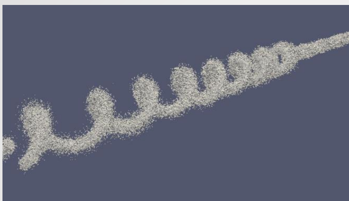
Fig 2: FM Voice, single transmission recorded by the Midwest Microwave Solutions SDR
