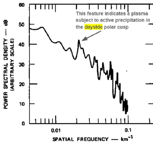
**Figure 1:** a) Chatanika ISR. b) Midnight auroral zone Chatanika ISR plasma density observations (contour interval is  $2e4 \text{ cm}^{-3}$ ). c) Associated irregularity spectrum developed using observations at 350 km altitude [Kelley et al., 1982].
