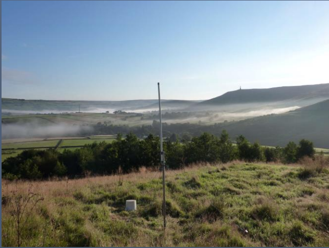
E-field Antenna Installed
