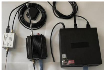
Figure 2: This picture shows the connections and basic layout of the PSWS System
