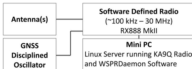
Figure 1: This diagram shows the basic layout of a PSWS System.
