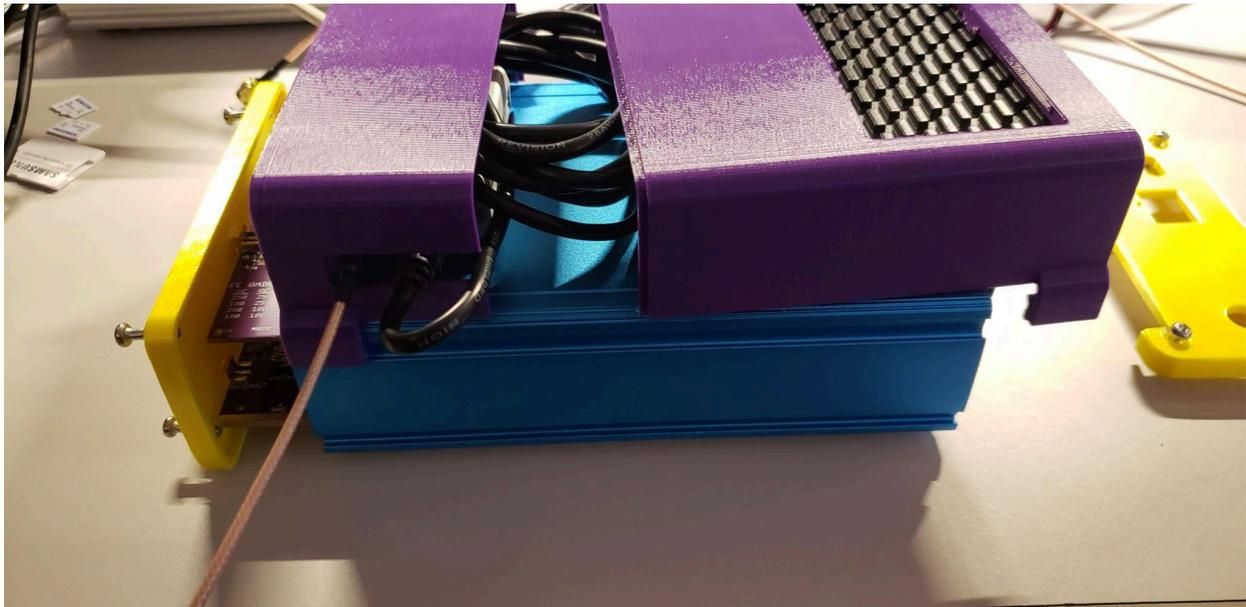
Once the jumpers are changed, reverse the above procedure and re-assemble the Grape2 unit back to the fully assembled unit. DO NOT overtighten the SMA connectors - they just need to be snug. Too tight will pop the snap ring holding the connector together and destroy it. Finger tight is sufficient for this connector re-torquing. You have been warned...
