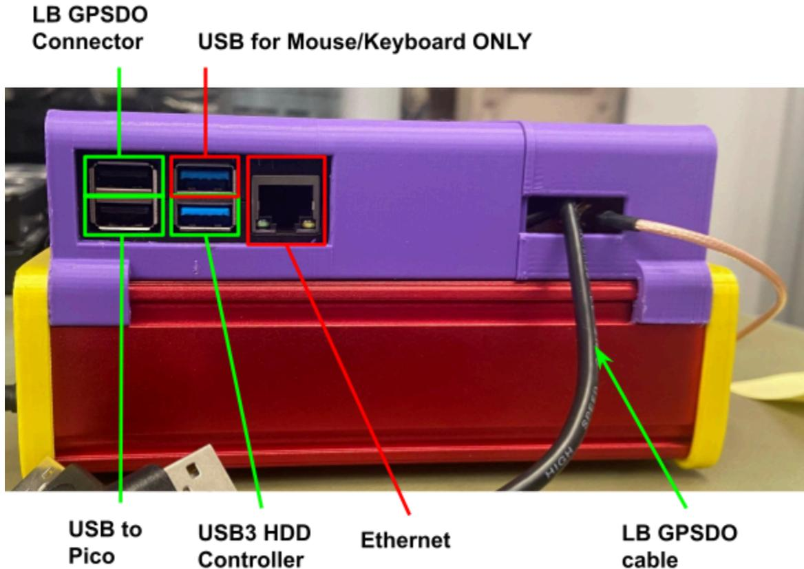
There should be three black cables physically attached to the unit, but not plugged in: the Leo Bodnar GPSDO connector (from the top box), pico connector (from the middle case), and hard drive connector (from the bottom hard drive controller). This is what it will look like connected:
