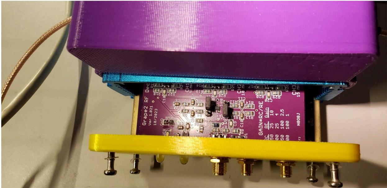
Position of whole assy during dis-assembly for Gain Jumper change procedure
