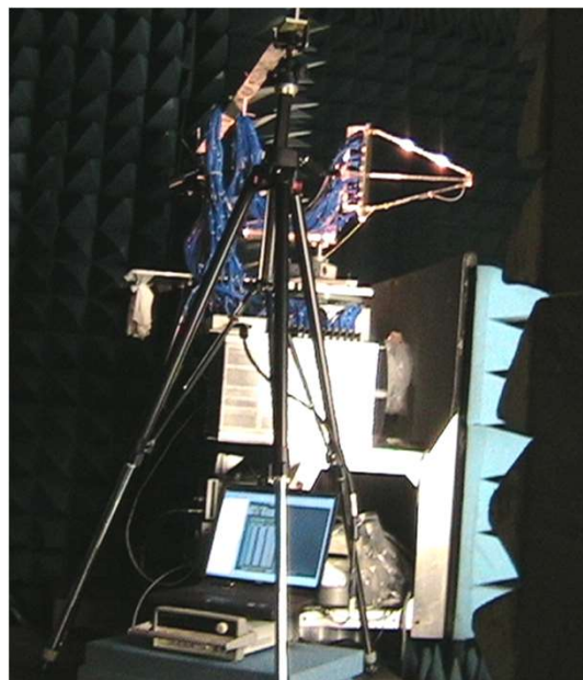
Testing the 615 Element K-band Reflectarray and Low Power Controller in NASA Glenn's Far Field Chamber
