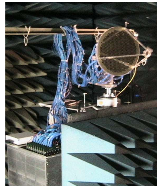
Testing the 615 Element K-band Reflectarray and Low Power Controller in NASA Glenn's Far Field Chamber
