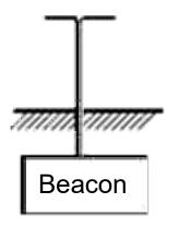
P = 800 Watts,  $\Delta P < 0.1 \text{ dB}$ f = 5.39 MHz,  $\Delta f < 5 \text{ Hz}$
